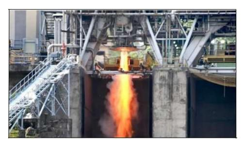
Isro has accomplished the human rating of its cryogenic engine (CE20), which powers the cryogenic stage of the human-rated LVM3 launcher for India's first human space flight mission Gaganyaan.
